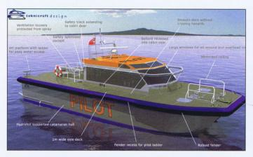
While foil assisted catamarans are not a new type of vessel for Q-West to construct, the Teknicraft Design catamaran currently under construction for Ports of Auckland in New Zealand is the first they have built specifically as a pilot vessel. In its specifications for a new pilot vessel, Ports of Auckland required a craft to meet its exacting pilotage requirements in all weather conditions, something its existing vessels are not always capable of.
