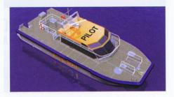
The 15-metre catamaran, which is under construction at Q-West Boatbuilders, features Teknicraft's low resistance, asymmetrical hull. It will be fitted with their adjustable hydrofoil system to ensure excellent fuel economy and ride comfort for the pilots.
